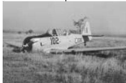
remained until the machine was moved out. The major concern was that there might be a fuel leak which could lead to a fire. The wings of the Harvard were detached and the whole aircraft was loaded onto an air-force truck which transported it, via the ferry, back to the base for repairs.
